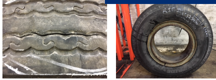
17-Channel Crack/Weather Check
